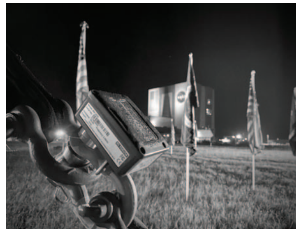
Figure 6 – Monitoring guy wire tension on an outdoor stage
