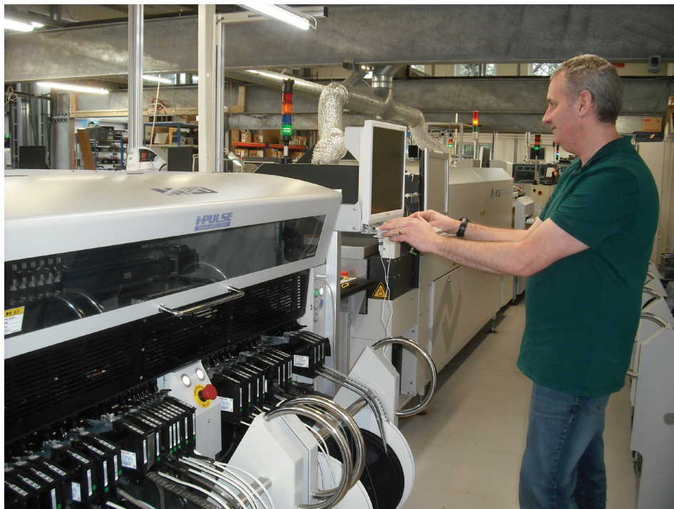
The Surface Mount Line in Mantracourt's factory. This machine places up to 26,000 components per hour.
