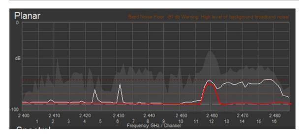
Whilst you are doing this, it is a very good idea to take screen shots of the whole window (the spectral view can give a useful history as well). This will be a useful record and could help with fault finding. It will also be useful to note down what the noise floor was as this could limit the possible range.
