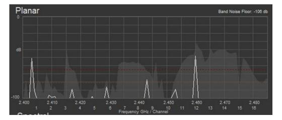
This shows a good RF environment. The Band Noise Floor is low and there are no red traces indicating that there are plenty of signal free gaps to enable BroadWeigh shackles to transmit. There is traffic across the whole band with higher signal traffic between channels 11 to 15, but there is nothing that would affect BroadWeigh operation.
