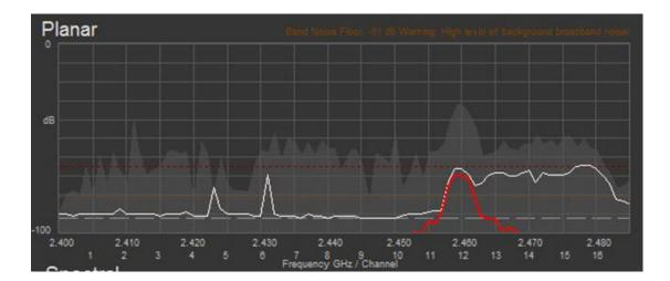
This shows how the display would look if the band noise floor slowly crept up. The red trace is only visible on channel 12 but other channels that were once OK (Having a very low minimum signal level) now have a viewable level of minimum signal noise. A double-click on the planar chart would reset the peak and minimum calculations so the minimum red trace would then follow the more recent higher noise floor – see image on next page.
